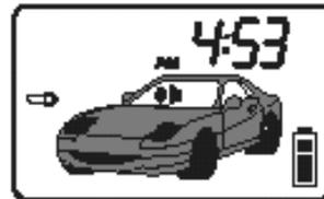
**Engine Run** indicates the engine is running on remote start equipped systems
