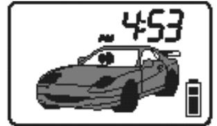
**Trunk Release** indicates the trunk or auxiliary function has been activated.
