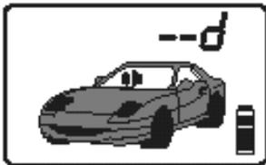
**System Armed** indicates the doors are locked and the alarm is on.
