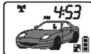
**Unlock** indicates the doors are unlocked and the system is in valet Code.
