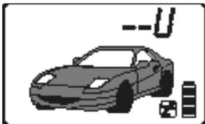
**Lock** indicates the doors are locked and the system is in valet mode.
