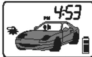
**System Disarmed** indicates the doors are unlocked and the alarm is off.
