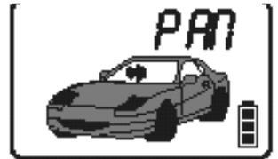
**Trunk Open** indicates the trunk or hood zone has been triggered.
